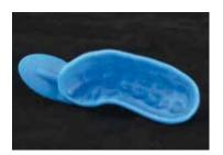
Partial tray printed in thick layers
