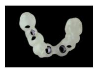
Dimensionally stable, steam-sterilised drilling template with accurate fit of drill sleeves
