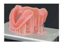
Additively fabricated denture bases
