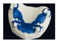
Printed model casting for fit check on the dental model
